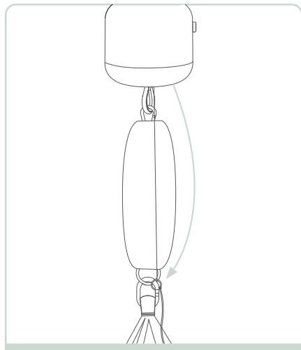
**5** Mounting the motor wire (on the outside of the spring bag)
