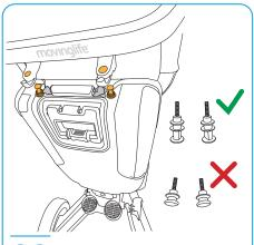
Unscrew the SHORT plastic knobs attached to the back. Replace them with the LONG knobs provided in the box. Then, place the holes of the orthopedic backrest over the knobs and make sure it sits firmly in place.
