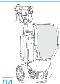
Folded mode: attach the orthopedic back to the back of the scooter back, with the long knobs.
