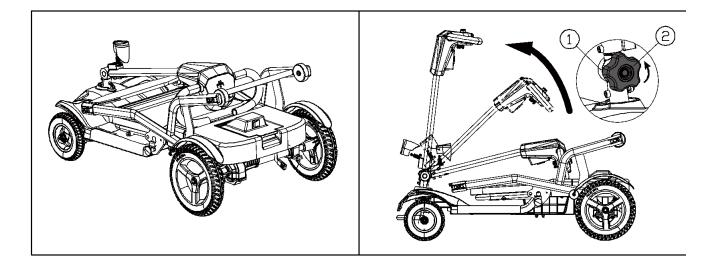
4.1.1.2 Pull the pin(③) out until it comes out of the hole, turn the seat backwards until you hear a "pop", then the pin is automatically locked into the hole, which means that the Ezylight is fully unfolded. (③ Pin)
