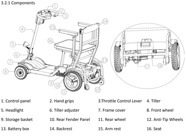
17. Transaxle Assembly 18. Manual Freewheel Lever
