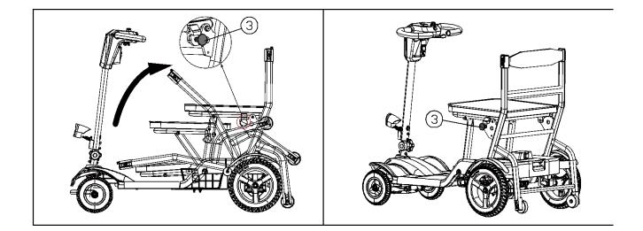
**Caution:** When unfolding, do not put your fingers into the scissors mechanism to avoid pinching your fingers.
