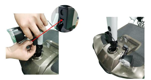
4.4.2.1 Hold down the dogging with one finger, pull the headlight upward with the other hand slightly, the headlight will be detached from the base.
