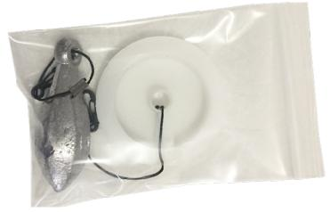
The **Throw Weight** bag actually contains two items. The first, a 10 oz lead throw weight with a carabiner for attaching to a paracord, is used to get your antenna up as high as you can throw over a tree limb. The second item, a spool and carabiner, is used for the Inverted-V antenna configuration to hold the antenna wire up without it touching the tree limb and thus losing significant power into the tree.
