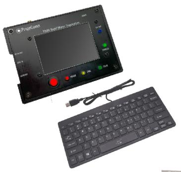
The star of the show is the **PreppComm MMX Multi-Band Morse Code Transceiver**. This comes with a small keyboard for entering the text you want to transmit, which is displayed on the color touchscreen. Incoming text is also displayed on the screen in a different color.
