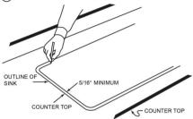
3 Cut on inside line. Cut straight front-to-back and left-to right
