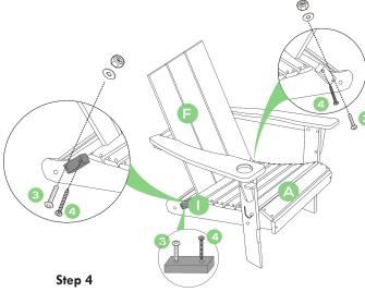
Attach the folding Bracket (Part I) per side Followed by attaching the Back (Part F) to the Seat legs (Part A)Use Qty: 1 of M6x50 Bolt & M6x50Screw (Part 3-4) per side.
