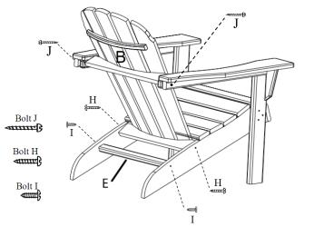
**STEP 2:** Attach the front part of the Arms (D) to the Front Legs (C) using 2.55" Bolts (H) and secure each with washer (G) and nut (F) as pictured.
