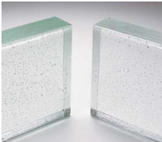
Tekta Clear, left, for cost savings. Tekta Crystal Clear, right, for crystal clarity, especially in thicker kilnwork. Blocks shown here are 8" x 8" x 1.75" (203 x 203 x 44 mm), fused from fourteen layers of 3 mm Tekta sheet.
