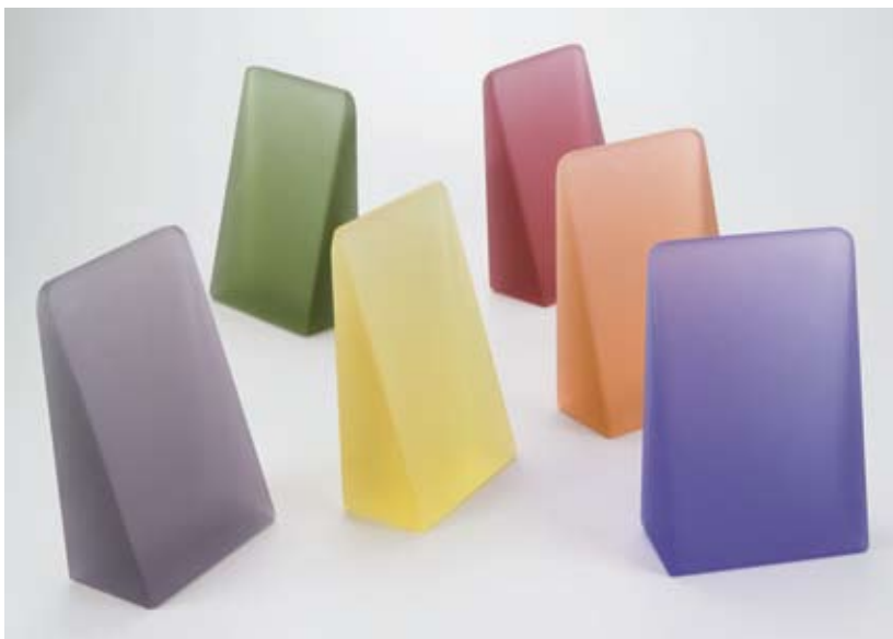
These cast and coldworked wedges show how the 001900 tint colors appear in thin and thick sections. Dimensions: 8.875 x 6 x 2.75 inches (each).
