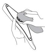
If dirt or dust gets in the terminal on the charger stand, carefully remove with a cotton swab or similar soft object. Do not use a metallic tool such as tweezers.
