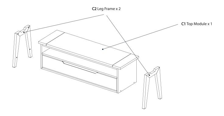
Step 2 - Attach Leg frames to the top module.
