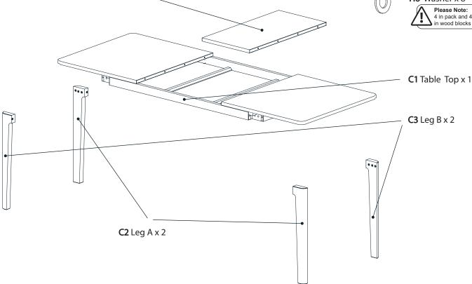
Remove 4 wedges from the Table top C1 by using an allen key (T2).
