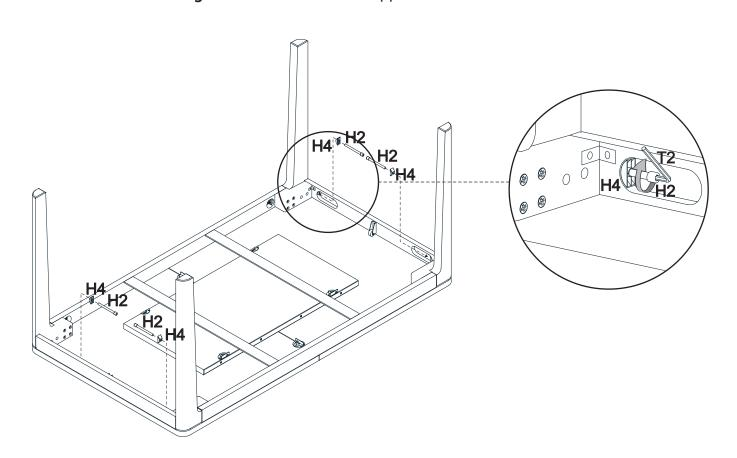
Step 6 - Fix the legs by using bolts.
