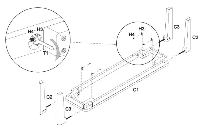
Step 4 - Fix the legs by using imbus bolts.
