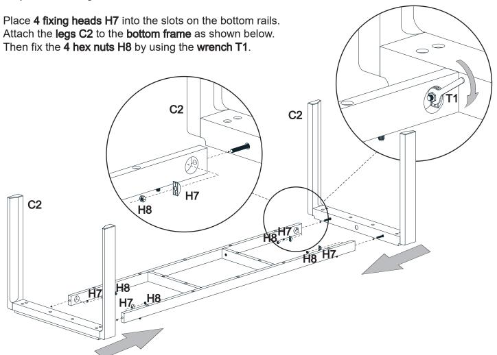
Step 8 - Fix the bottom frame and legs by using bolts.
