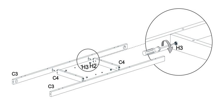
Step 5 - Attach wooden dowels to bottom frame.
