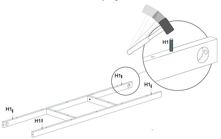
Step 6 - Attach headless bolts to leg frames.
