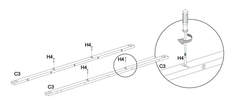
Step 4 - Attach barrel housings to bottom rails.
