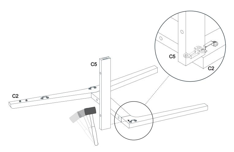
**Step 3 -** Attach the **second cross rail C5** to the **leg frame C2** as shown below.
