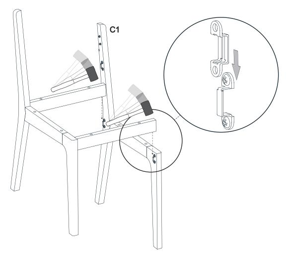
Step 5 - Install back rest B C4 as shown below.
