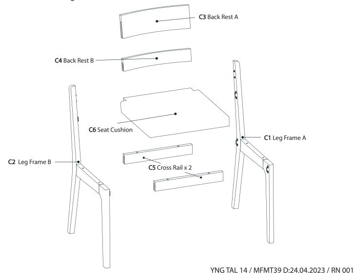
Step 2 - Attach the first cross rail C5 to the leg frame C2 as shown below.
