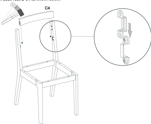
Step 6 - Install back rest A C3 as shown below.
