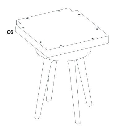
**Step 8 -** Place the chair on the seat cushion. Install **8x bolts H1** as shown below. Tighten them by using **allen key T1.**
