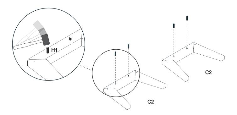
Step 3 - Attach the first leg frame to the main module.
