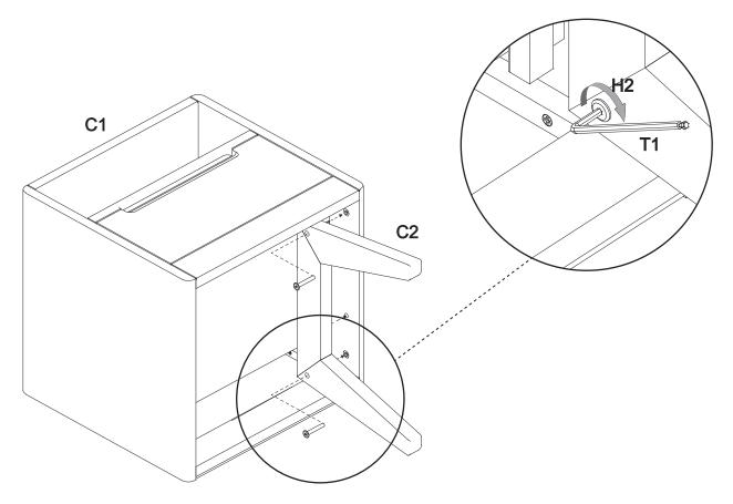
Step 4 - Attach the second leg frame to the main module.
