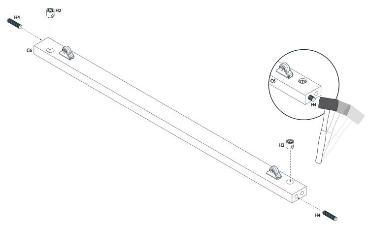
Step 7 - Attach wooden dowels to bottom support (sides).
