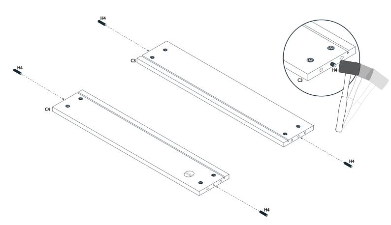
Step 6 - Attach wooden dowels and barrel housings to bottom support (middle).
