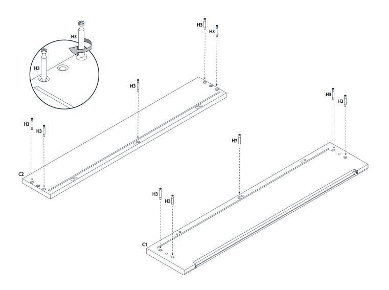
Step 4 - Attach barrel housing to left and right panels.
