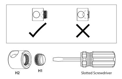
Step 3 - Attach Steel Dowels to front and back panels.
