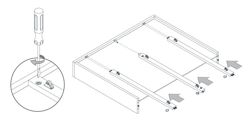
Step 11 - Attach the front panel.
