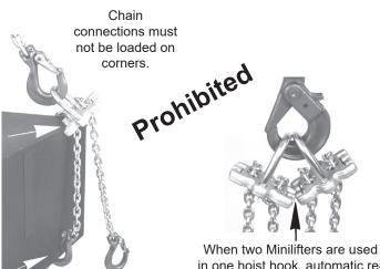
Load hooks must not be loaded on the tip.
