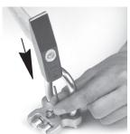
Hammer clamping sleeve out with drift punch
