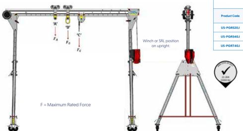
Where Maximum Rated Force is 22.2 kN [5000lb] the product is tested and meets the requirements of ANSI 7359.18 for 1 user. Where Maximum Rated Force is less than 22.2kN [5000lb] OSHA Regulations apply - miumum safety factor of 2:1. All trollies and sheave carriers are ANSI 7359.18 rated for one user.
