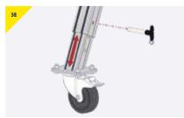
The foot option can be changed by removing the ball lock pin and withdrawing the foot cartridge assembly
