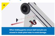
> To fold the gantry reverse steps 10 to 1 for Standard Assembly or steps 27 to 23 for Confined Space Assembly
