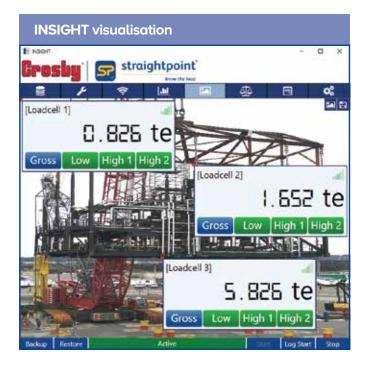
INSIGHT software, supplied with an SW-D USB wireless dongle, allows connection of up to 126 Straightpoint wireless load cells simultaneously onto any Windows tablet or laptop.
