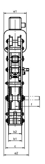
f = required space for removing brake shoe pin
