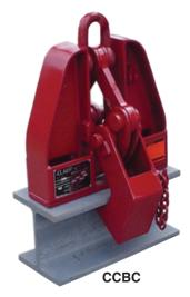
Crosby Clamp-Co® Beam Clamps provide an efficient method for handling wide flange beam sections and plate girders. When lifting, these beam clamps grip the beam at three points, and when properly balanced and safely guided, the beam can be handled even if the clamp is slightly off center lengthwise.
