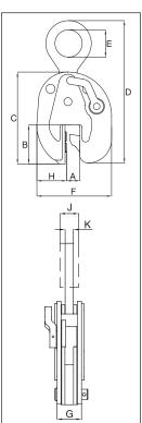
Model IPSBUUZ and IPSBUSUZ: With Universal Hoisting Eye Model IPSBUZ and IPSBUSZ: With Fixed Hoisting Eye
