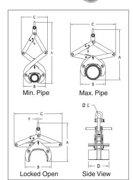
The new Crosby Clamp-Co® Adjustable Pipe Grab provides an excellent means of handling cylindrical objects. Featuring padded grabs, the new Grab offers an excellent method of handling any pipe or solid bar, 3.5" to 36", especially where damage to material surface is not permitted.
