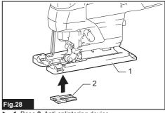
▶ 1. Base 2. Anti-splintering device
