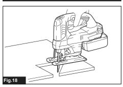
To trim edges or make dimensional adjustments, run the jig saw blade lightly along the cut edges.
