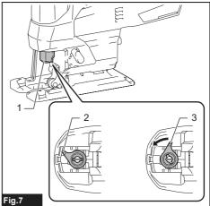
1. Jig saw blade holder 2. Blade clamp lever (released position) 3. Blade clamp lever (fixed position)
