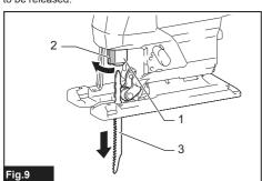
1. Jig saw blade holder 2. Blade clamp lever 3. Jig saw blade
