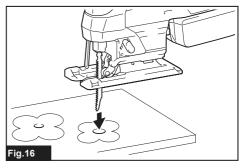
For internal cutouts without a lead-in cut from an edge, pre-drill a starting hole 12 mm or more in diameter. Insert the jig saw blade into this hole to start your cut.
