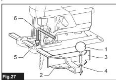
1. Threaded knob 2. Fence guide 3. Rip fence (Guide rule) 4. Circular guide pin 5. Bolt 6. Hex wrench
