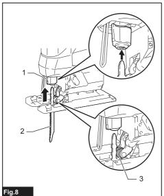
▶ 1. Jig saw blade holder 2. Jig saw blade 3. Roller
