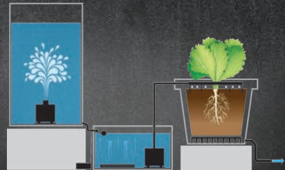
Run to waste system
