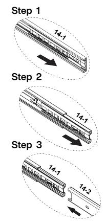
Before installation, slide the inner iron pieces of #14-1 to the outermost side. Then align it with #14-2 and gently push it inward to complete the slide installation.
