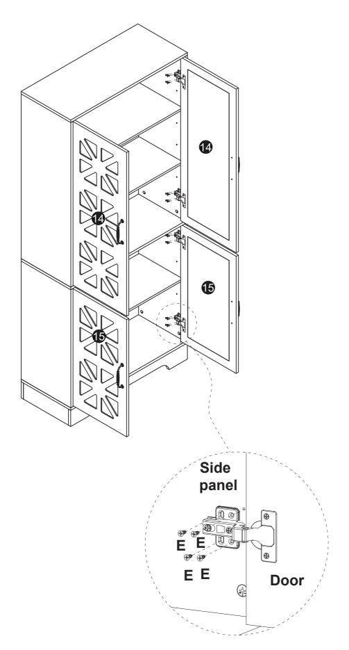
To prevent the door hinge from falling off,please install 4 screws
