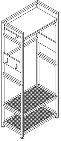
Notes: Don't tighten screws completely at first, just in case parts were assembled wrong and need disassemble. Tighten screws at last when all parts are put together
