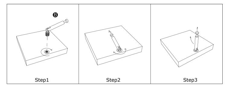
Screw the pin into the hole. Set the cams correctly by aligning the head of the cams with the lock pins. Lock the cam by turning the cam head with a screwdriver until it is tightened. Please do not use an electric screwdriver to assemble the unit.
