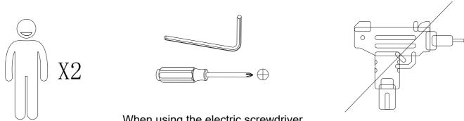
When using the electric screwdriver, Reduce the power and torque to avoid damaging the furniture
