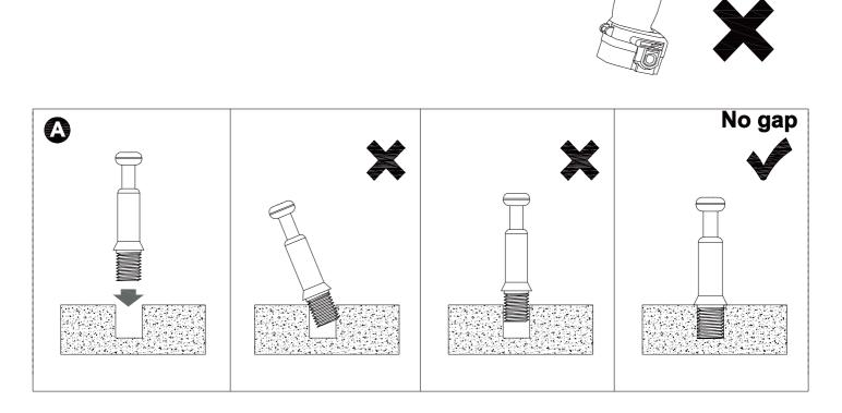
Screw the pin into the hole. Set the cams correctly by aligning the head of the cams with the lock pins.Lock the cam by turning the cam head with a screwdriver until it is tightened. Please do not use an electric screwdriver to assemble the unit.
