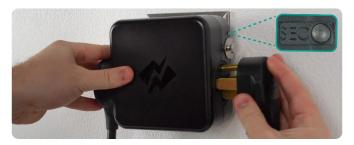
If you are using an extension cord with your Smart Splitter, please ensure the cord is UL certified and is the proper gauge wire.
