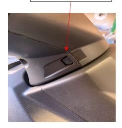
Unscrew the ride system trigger and remove from bars
