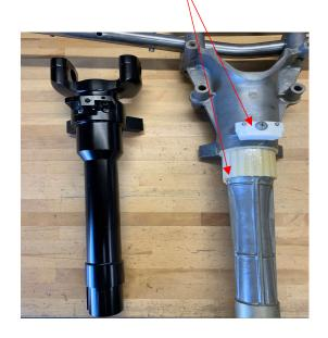
Grease Pivot points on new stem. Fit WORX Steering stem into OEM location. Make sure OEM bush located in housing.
