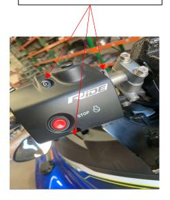
Unscrew throttle trigger and remove from bars
