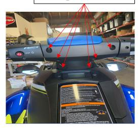
Push tab in to fully pull bar pad off
