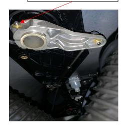
Transfer OEM bushings and magnet onto WORX stem
