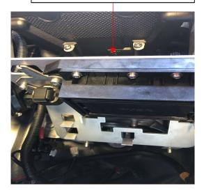
Install the breather filter (WR04020-6) to the breather hose. Mount Breather high in the engine bay, do not twist or restrict this hose.
