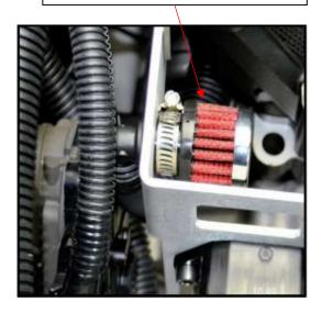
10 Install throttle body adapter (WR04043) and air filter element
