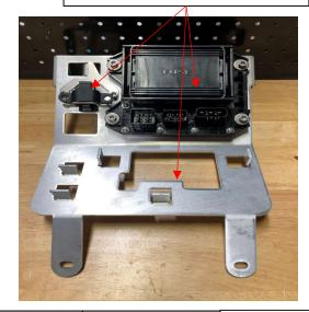
Fuse Box Holder 4 x M6 x 30 cap 4 x M6 washer 4 x spacer 4 x ¼ x ¾ washer Bracket mount 4 x M8 x 20 cap 4 x M8 spring washer 4 x M8 washer Angle sensor 2 x M6 x 16 cap 2 x M6 washer 2 x M6 nut
