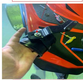
11 Install the Flexible hose to the supercharger adapter
