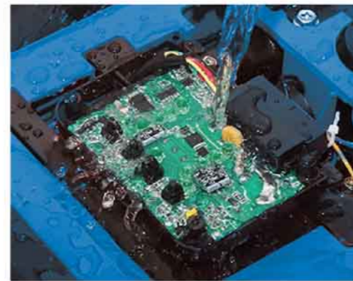
Circuit board gumming process waterproof and moisture proof
