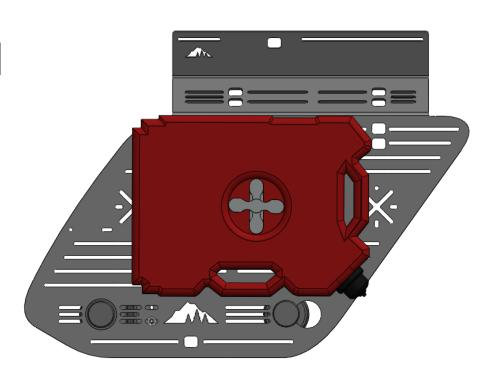
Once the Rotopax container is situated, lift it back off of the panel slightly and install the supplied vibration dampening plugs through the slots in the four corners of contact between the container and the panel.
