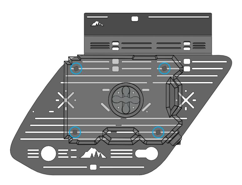
Repeat the installation process in the two outer Rotopax mounting locations on the panel if you plan to use 2x 2 gallon containers, or 1x 4 gallon container.
