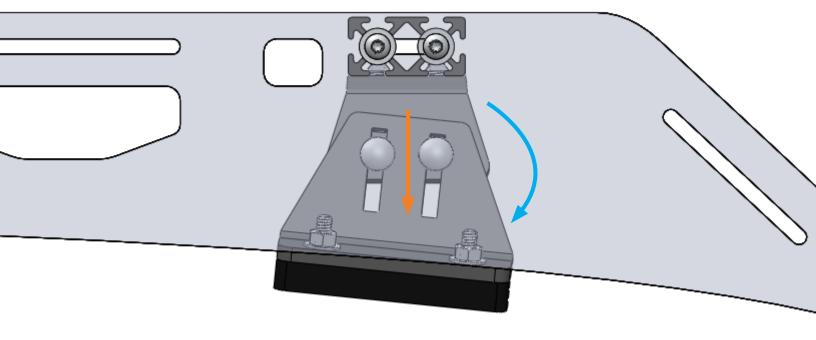
Final adjustments can be made to the front leveling mounts once the rack has been assembled on the vehicle. We recommend an extra set of hands for this step. You may also need to loosen the middle mounts for this step depending on your configuration.
