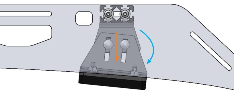
Final adjustments can be made to the front leveling mounts once the rack has been assembled on the vehicle. We recommend an extra set of hands for this step. You may also need to loosen the middle mounts for this step depending on your configuration.
