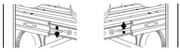
The shelves are removable to help with cleaning and maintenance. To remove a shelf, pull it out as far as you can. There are levers on each side of the shelf near the rollers. Left the lever on the left hand side and push down the lever on the right hand side to remove the shelf from the tracks.
