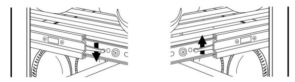
The shelves are removable to help with cleaning and maintenance. To remove a shelf, pull it out as far as you can. There are levers on each side of the shelf near the rollers. Lift the lever on the left hand side and push down on the lever on the right hand side to remove the shelf from the tracks.
