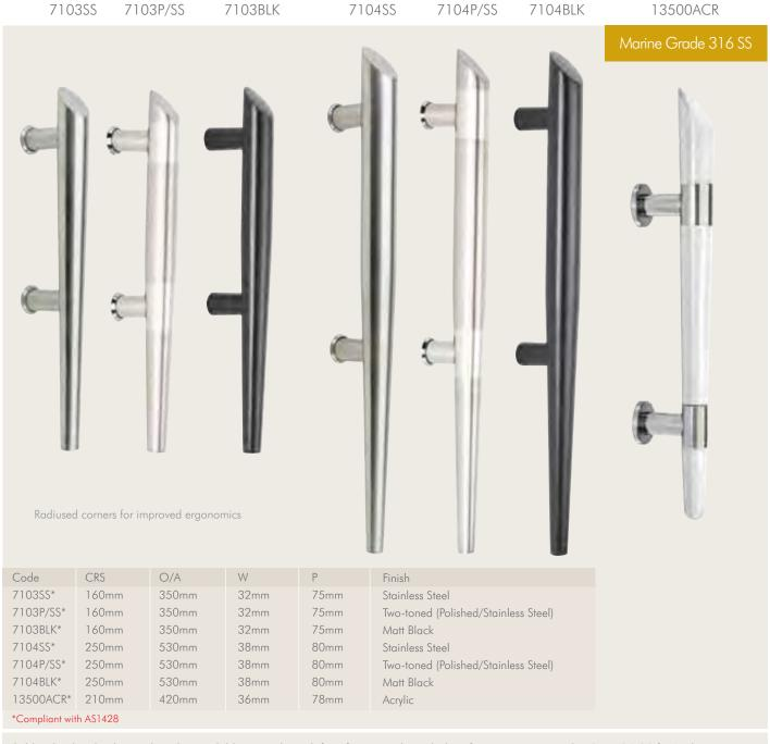
Sold as back to back pairs but also available as singles with face fix or rear through door fixing.
