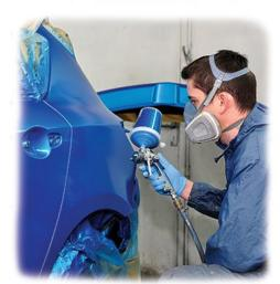
Features: Ideally suited for hot/dusty work settings that require long periods of wear. At least 95 percent filtration efficiency against certain non-oil based particles. 3M™ cool flow™ exhalation valve reduces heat build-up inside the respirator. Braided headbands, Spacious & durable. Designed to increase comfort and wearability. Advanced electret media designed for ease of breathing.
