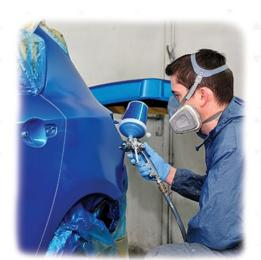
**Features:** Exceptional 99.97% filter efficiency meets NIOSH P100-series test criteria. Versatile protection against many oil & non-oil based particulate contaminants. Nuisance odor relief for organic vapor levels below the permissible exposure level (PEL). Bayonet compatibility allows use with many 3M™ half & full facepiece designs. Wide range of applications reduces inventory needs & training requirements.
