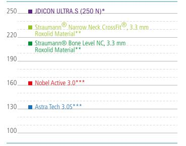
Fatigue strength is the maximum force an implant / abutment structure can survive for at least five million cycles. JDIcon Ultra.S has been tested according to ISO 14801 that is accepted by many regulatory agencies including FDA and Notified Bodies (CE).
