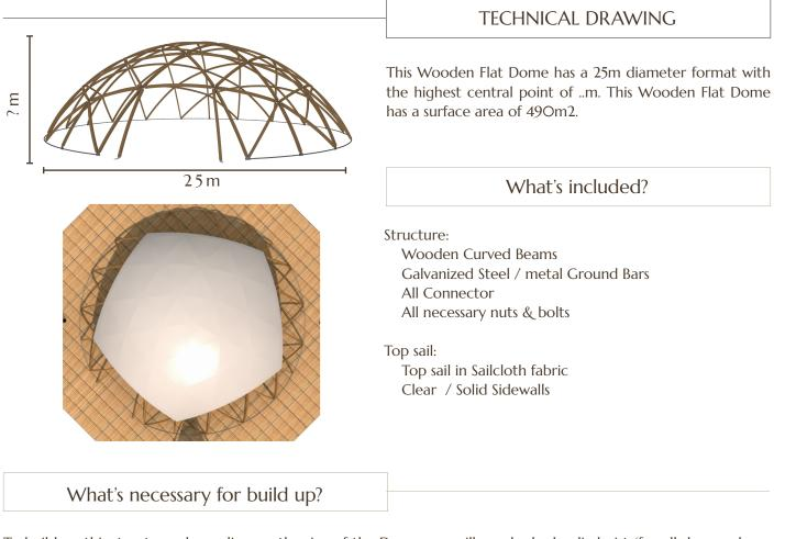
To build up this structure, depending on the size of the Dome you will need a hydraulic hoist (for all domes above 20m diameter) and two sets of scaffolding (6Hx2L m). A build up manual will be provided after the purchase of this tent structure.
