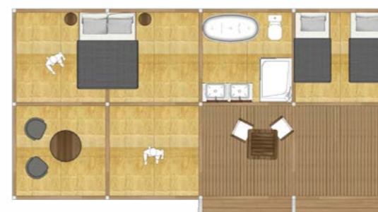
The internal space can be re-configured by clipping internal walls to different points on the frame.
