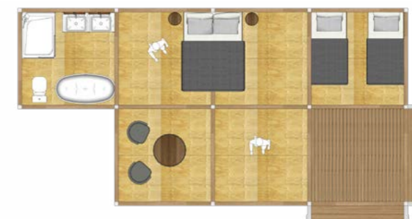
The internal space can be re-configured by clipping internal walls to different points on the frame.
