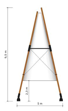
The Bamboo Tipi is 9.5 m high and the base is 5m x 5m. The cone is 7 m high and starts at a height of 2.3m.
