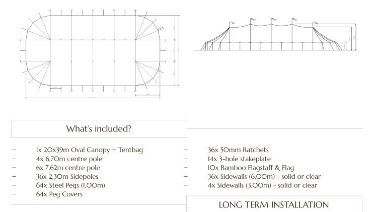
For (semi-)permanent builds we recommend adding baseplates under the poles for extra protection. This will greatly increase your pole's lifespan and structural integrity. For this tent, you will require following quantities (not included in a standard set):
