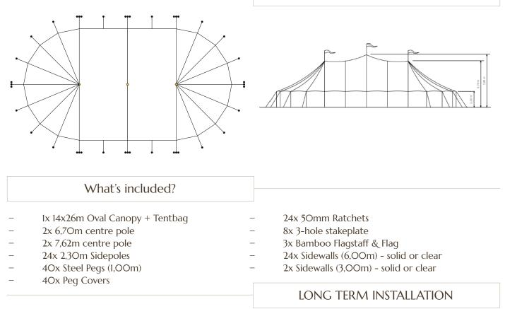
For (semi-)permanent builds we recommend adding baseplates under the poles for extra protection. This will greatly increase your pole's lifespan and structural integrity. For this tent, you will require following quantities (not included in a standard set):
