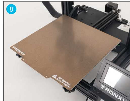
8 PEI magnetic sticker installation completed
