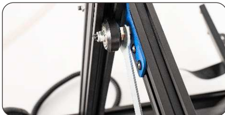
Use wrench to adjust the tightness of eccentric nut
