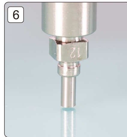
Fine tune to almost touch the platform 微调至几乎碰到平台
