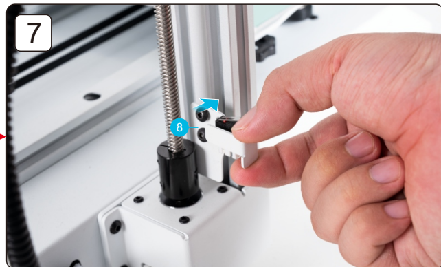
Install the Z-axis limit switch as shown in the figure 如图所示安装Z轴限位开关
