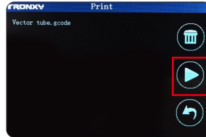
Confirm to print the document and click the "start printing" icon 确认打印文件, 点击“开始打印”图标
